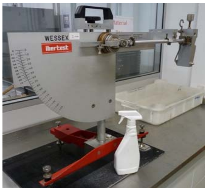
Figure 3 : Pendulum test equipment
