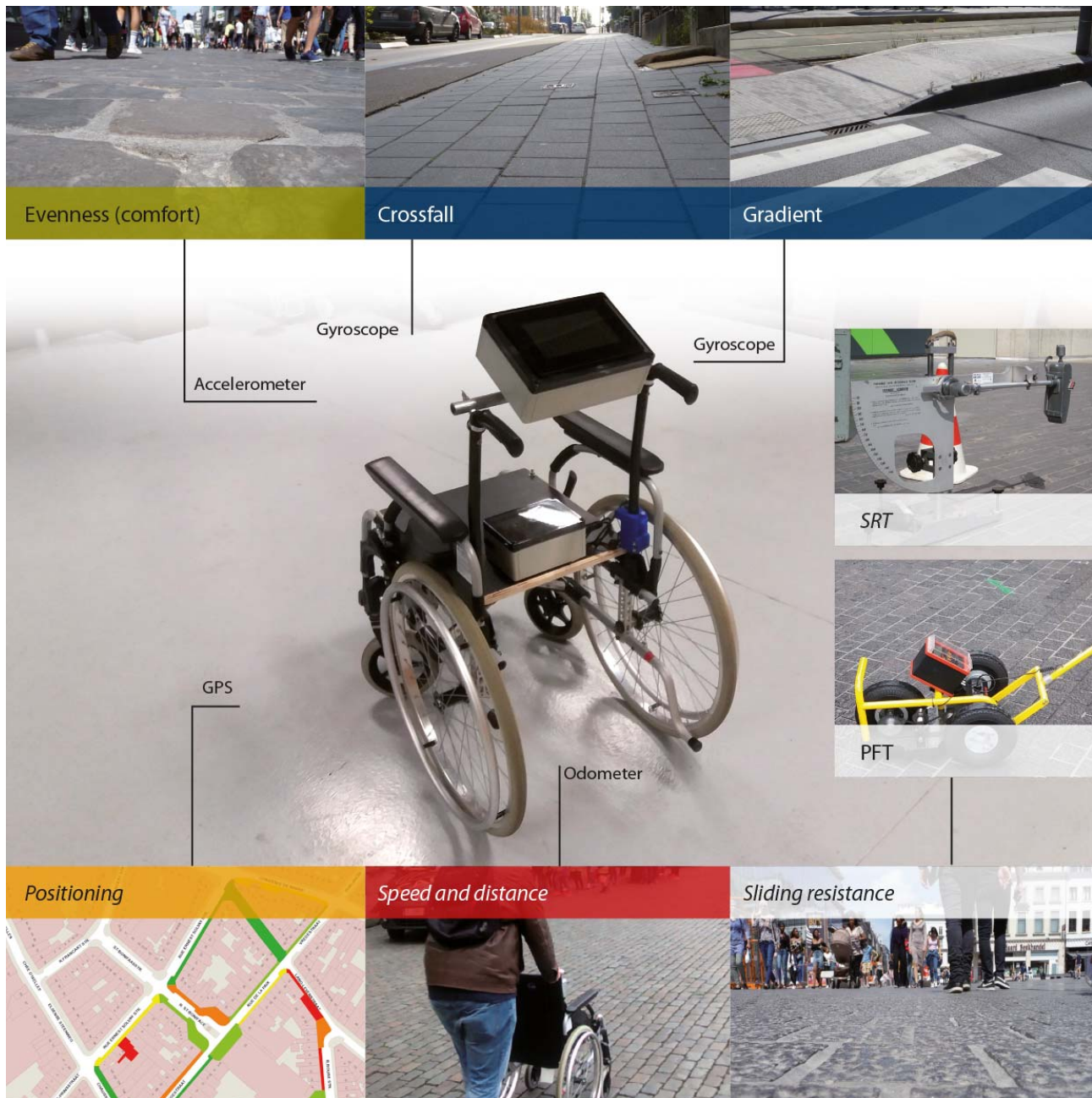
Fig.4. Tool for measuring the quality of use of pedestrian coatings under development (prototype 2) Source: BRRC
