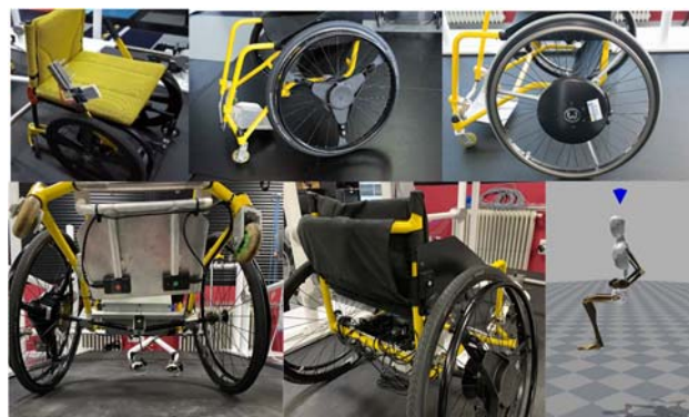
Figure 10: Vibration recording system in an instrumented wheelchair.
