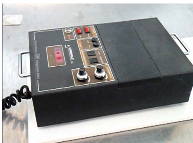
Figure 5 : Pull-off (SCOF) test equipment
