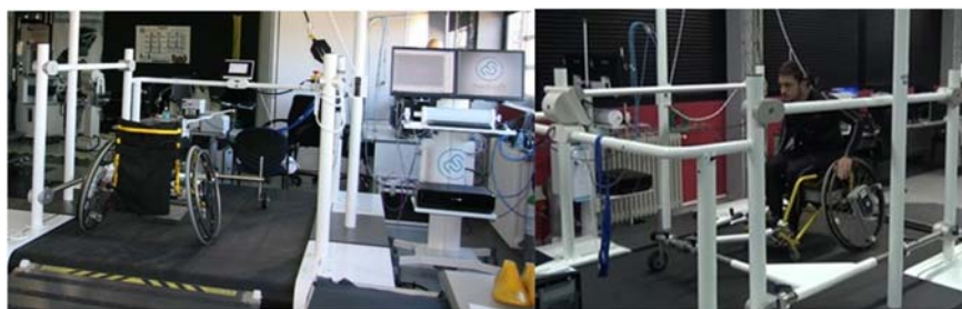
Figure 11: Treadmill integrated with ergospirometry system for wheelchair user evaluation.
