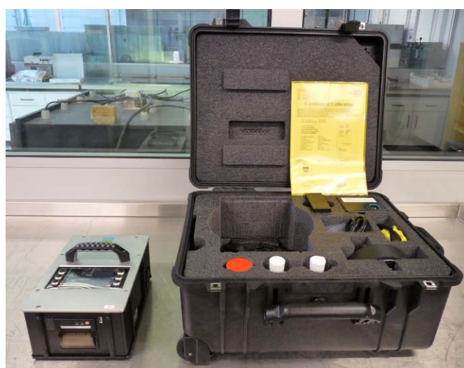
Figure 4 : BOT 3000 (DCOF) test equipment
