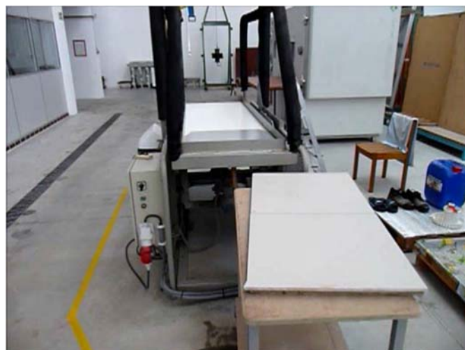
Figure 2 : Ramp test equipment
