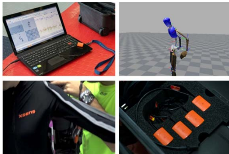
Figure 3: Xsens system based on IMUs technology.
