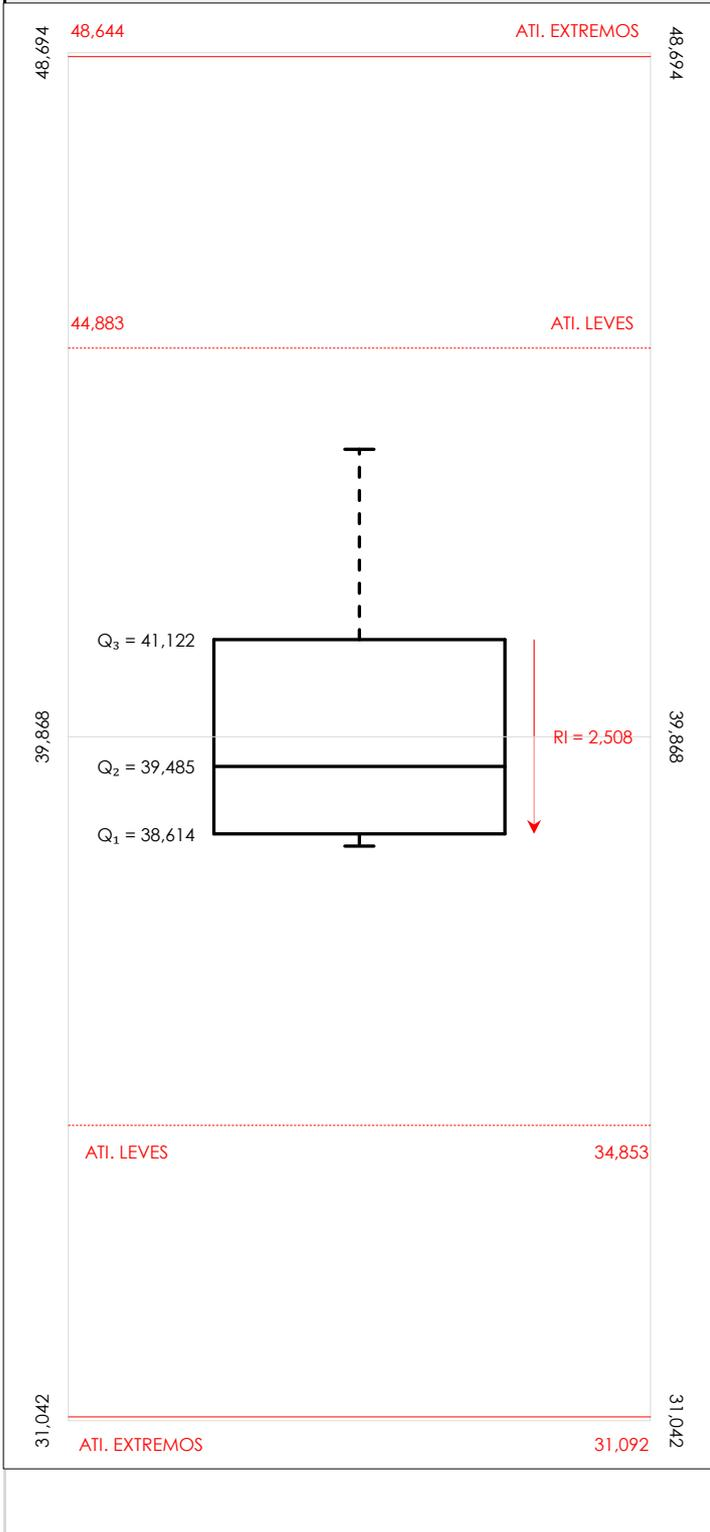
Diagrama Box-Plot post-estadístico. Eje Y: resist.compresion 28 d.cúbicas (N/mm<sup>2</sup>)
