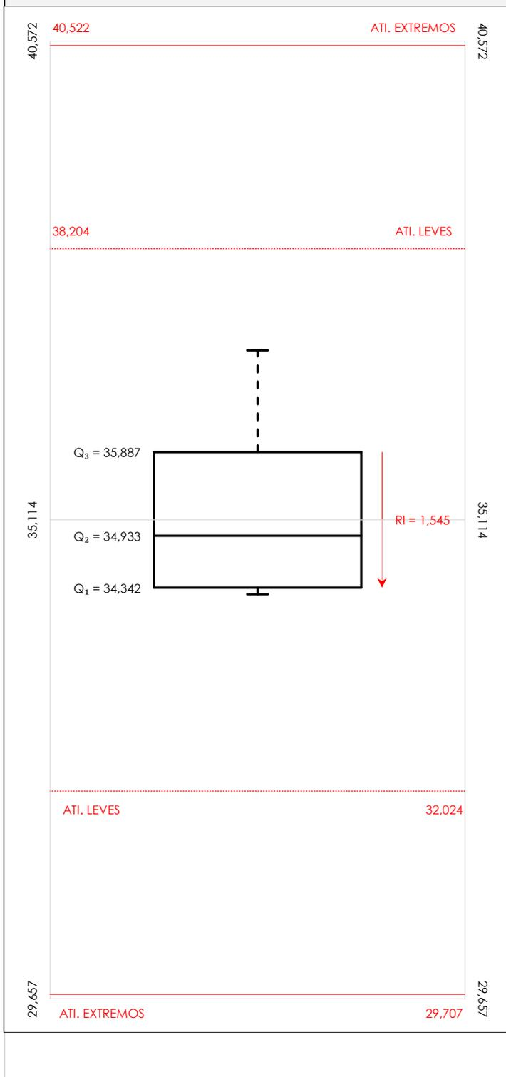
Diagrama Box-Plot post-estadístico. Eje Y: resist.compresion 28 d.cilindricas (N/mm<sup>2</sup>)
